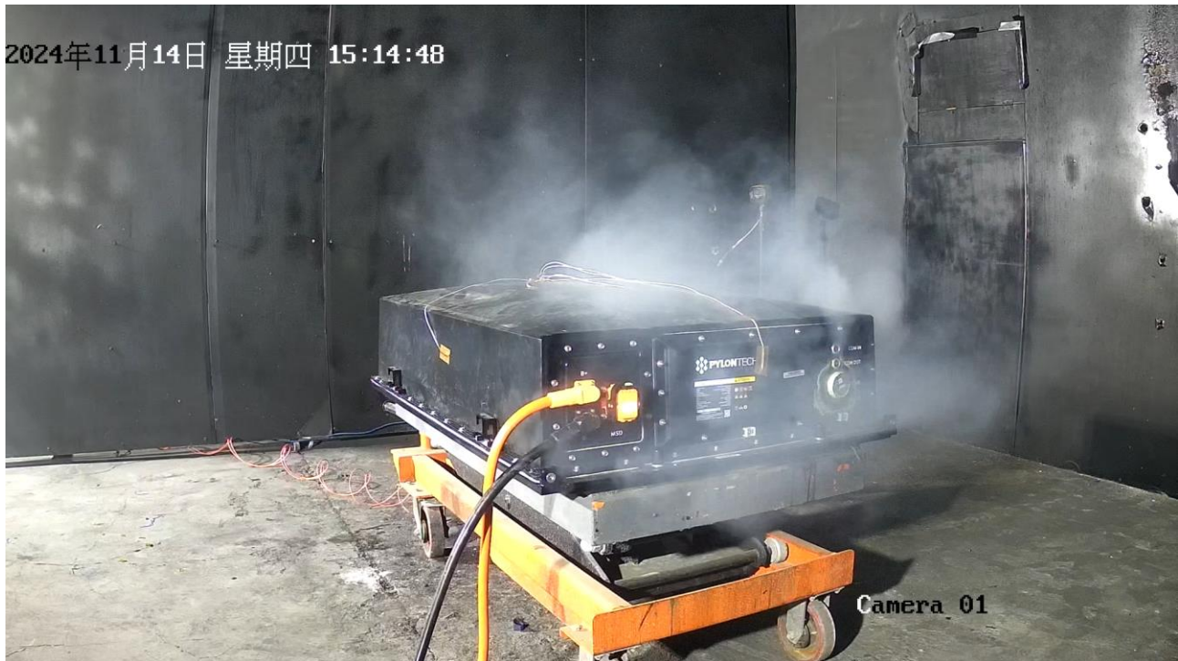
Figure 20. Smoke release during test
