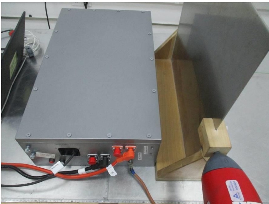
Photograph 3: Set-up for immunity test of electrostatic discharge
