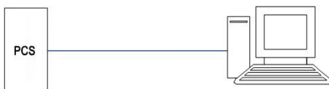
Fig. 6-9 Schematic diagram of single PCS Ethernet communication scheme
