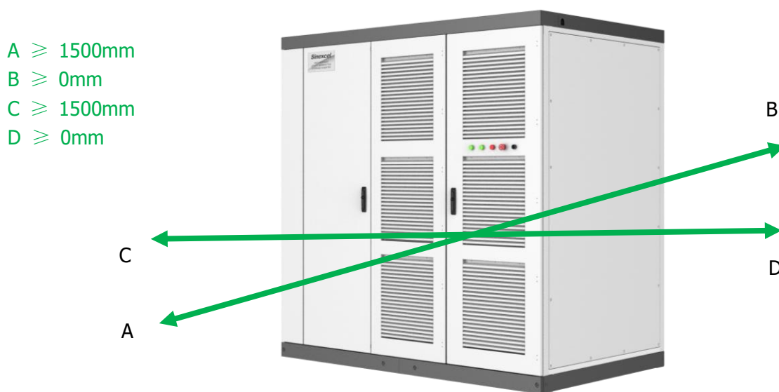
Fig. 6-2 Space requirements for energy storage converter
